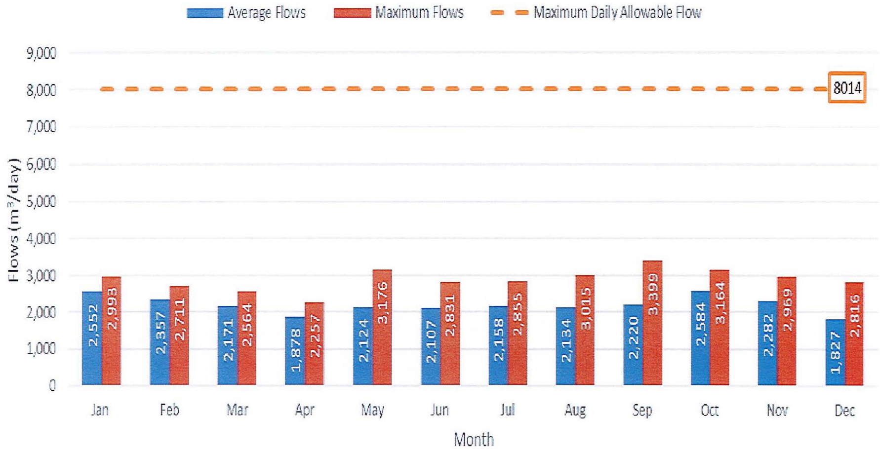
Comparison of the Average and Maximum Flow Rates for the Alexandria Drinking Water Treatment Plant
