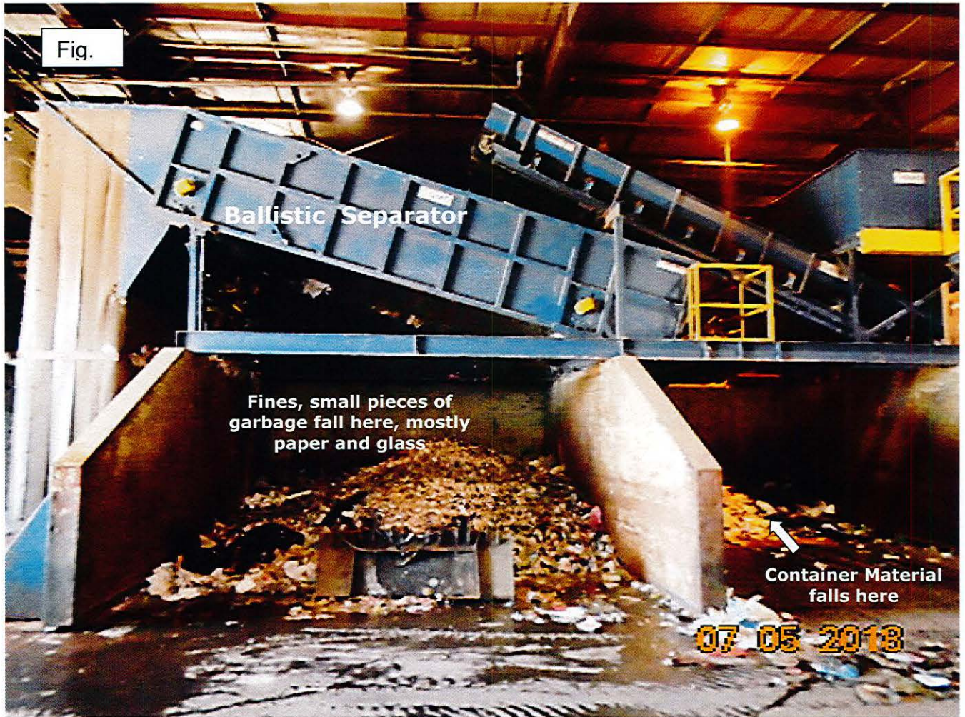
The Ballistic Separator must be removed to accommodate a dual stream system as the containers will fall away from the sorting stream and will need to be returned to the infeed conveyor for processing.
